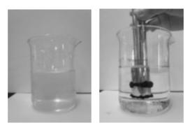
Figure 1: Water Purification by Magnetic Flocculant
